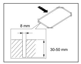
For installation of the loop cable use the number of turns indicated in the table.
